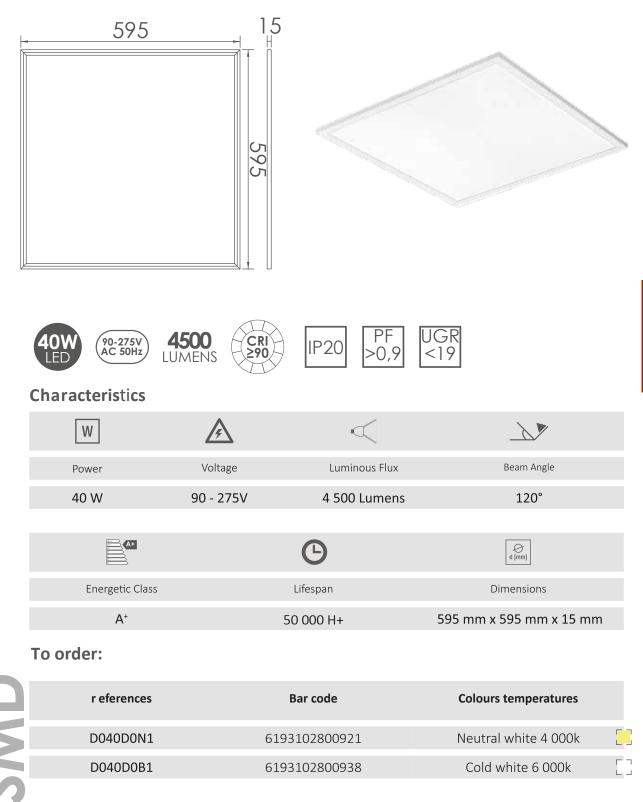
Surface mounting, suspended and recessed kits sold in option. Dimming : Dimmable Driver 0/1 to 10 optionnal
